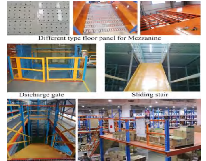
Mezzanine rack basic structure 阁楼式货架基本结构
