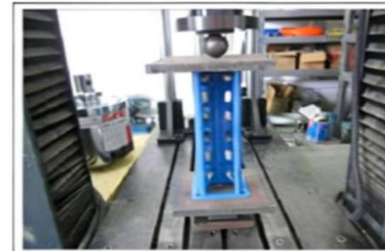
Before Stub column compression test
