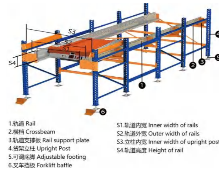
Radio shuttle rack structure details 穿梭式货架结构
