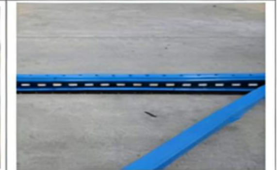
After Compression test on uprights
