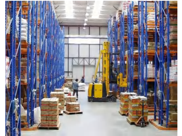
VNA rack project 窄巷式货架案例
