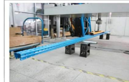
Before Bending tests on upright sections
