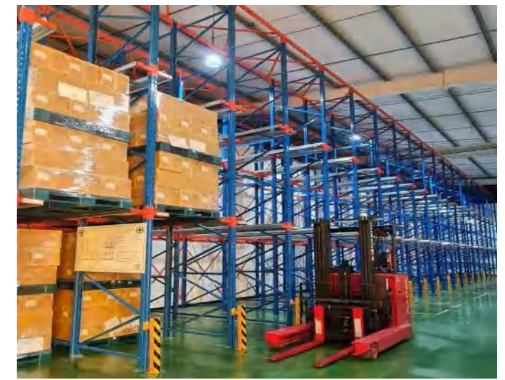
Drive-in rack project 驶入式货架案例
