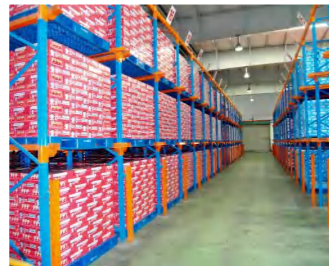
Drive-in rack project 驶入式货架案例
