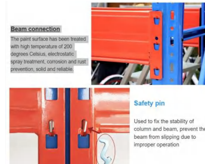
Structure details of racks 货架细节图
