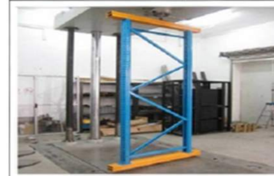
Before Compression test on uprights
