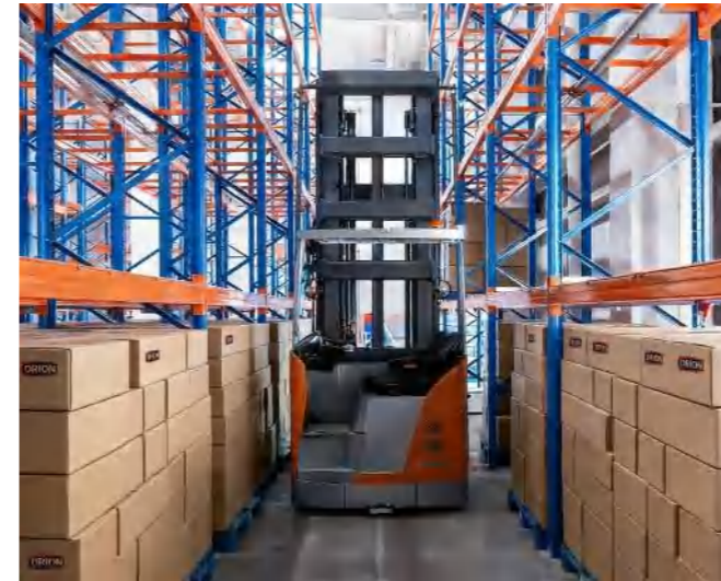
VNA rack project 窄巷式货架案例
