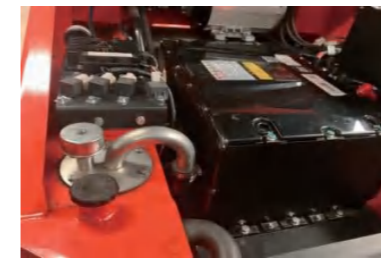
Easy inspection of hydraulic oil level. 液压油位方便检查
