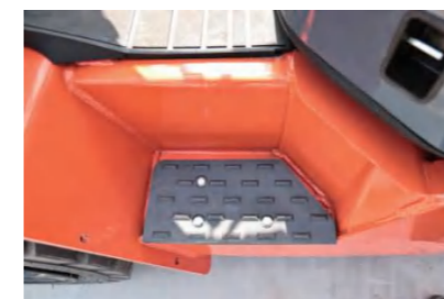
Enlarged boarding step 增大上车踏板
