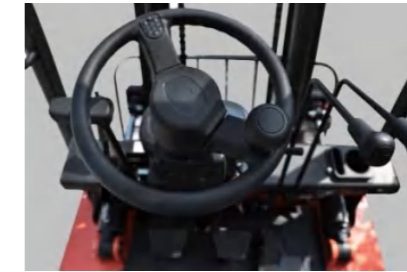
Smaller steering wheel reduces operator fatigue. 采用直径较小方向盘，减少了操作员的疲劳强度
