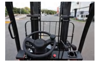
Wider mast for better visibility. 门架加宽，视野更佳
