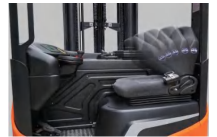
High-elasticity shock absorbing seat 高弹性减震座椅
