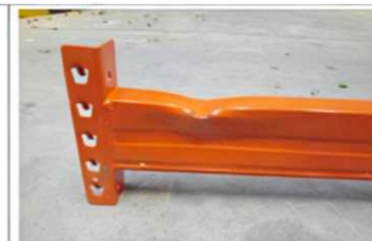
After Shear test on beam end connectors and connector locks
