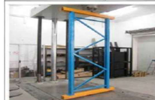
Before Compression test on uprights
