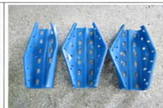
After Stub column compression test
