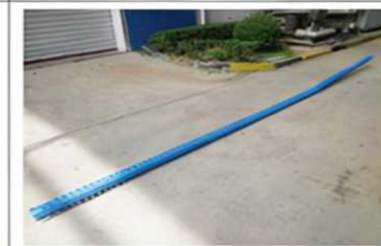
After Compression tests on uprights
