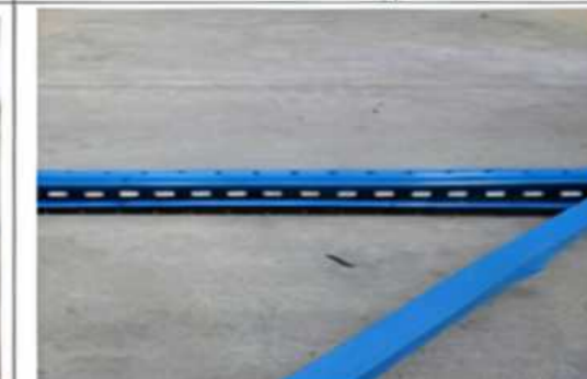
After Compression test on uprights
